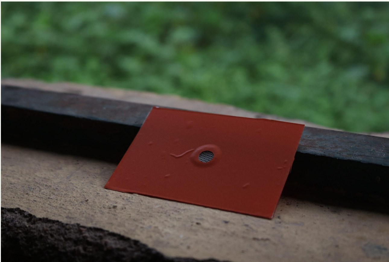
SchistoFilter - A Foldscope-compatible, reusable urine filter for schistosomiasis diagnostics in the field
